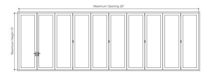
Bifold panel sizes range from 14-1/4" x 48" to 42" x 117-3/8". Using 10 door panels, the maximum opening is 26'.
